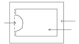
To remove the negative, gently push from left side to separate negative from cassette at the tab, then grab edge and pull back toward the left to remove completely. Touch the negative on the edges only, and as little as possible.
